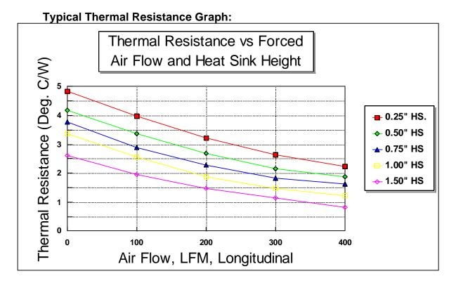
This graph shows how much the thermal resistance decreases with the amount of air flow and the height of the heatsink, for a typical natural convection extruded heatsink being used with forced air. Special heatsink construction techniques, such as bonded fin types or high fin density extrusions, can produce much better results.
